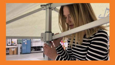
Standing again by the tent leg with your foot on the foot pad (as in Step 5), extend the leg by pressing the push button in and pulling up on the leg until it snaps into place. Repeat for this leg until you have reached desired height. Repeat for remaining three legs.
