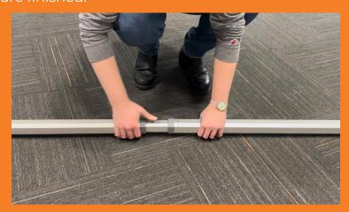
Lift the "X" frame pieces and latch the steel hook. It will sit above the point of connection.
